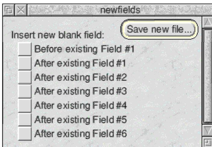
As with the main window, the vertical size of this window and the number of icons it will have depends on the loaded CSV/TSV file. In the case shown in the above screen-shot the loaded file has 6 fields per record. The top option icon is to add a new field **before** the existing first field, and this is followed by a number of option icons to add new fields **after** each of the existing fields - here, 6 such option icons, giving a total of 7 option icons.
