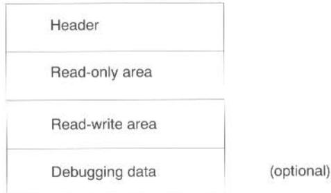
At this stage a debugger is expected to copy any debugging data to somewhere safe, otherwise it will be overwritten by the zero-initialised data and/or the heap/stack data of the program. A debugger can seize control at the appropriate moment by copying, then modifying, the third word of the AIF header (see *AIF Header Layout* on page 226).
